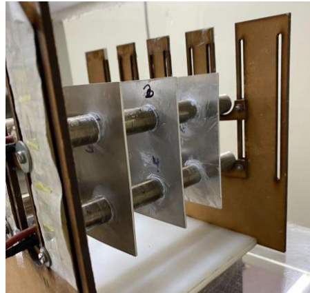
Figure 5. Holding structure and finned tube heat exchanger in the test section.
