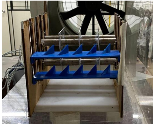
Figure 7. Vortex generator and heat exchanger assembly.
