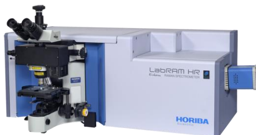
Figura 4. Microscópio Raman LabRam HR Evolution (HORIBA Scientific, 2022)
