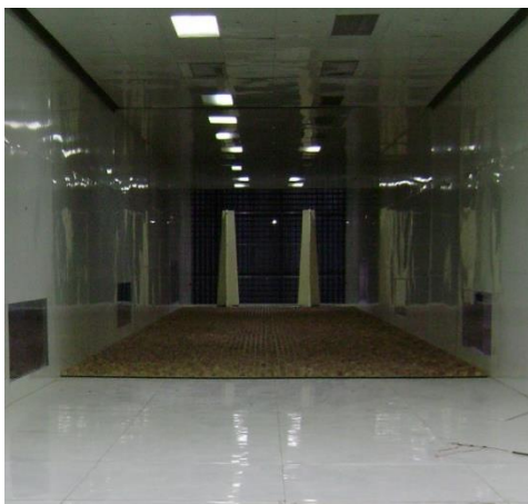
Figure 3. Hardware of turbulent flow simulation and vertical profiles of mean velocity and turbulence intensity.
