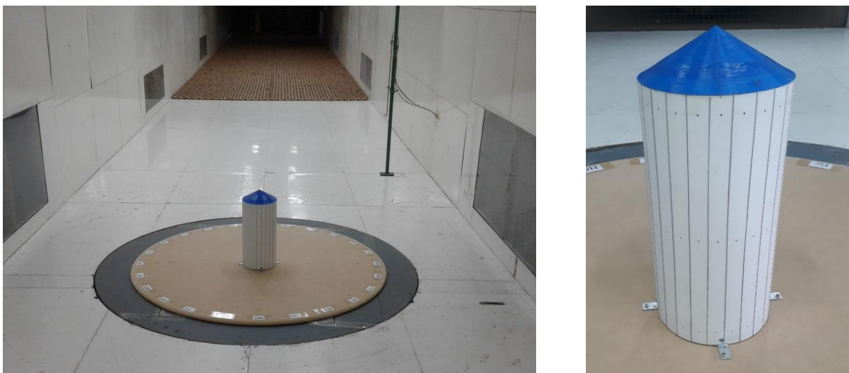
Figure 5. Model instrumented in the wind tunnel test section and details of the rough surface silo model.
