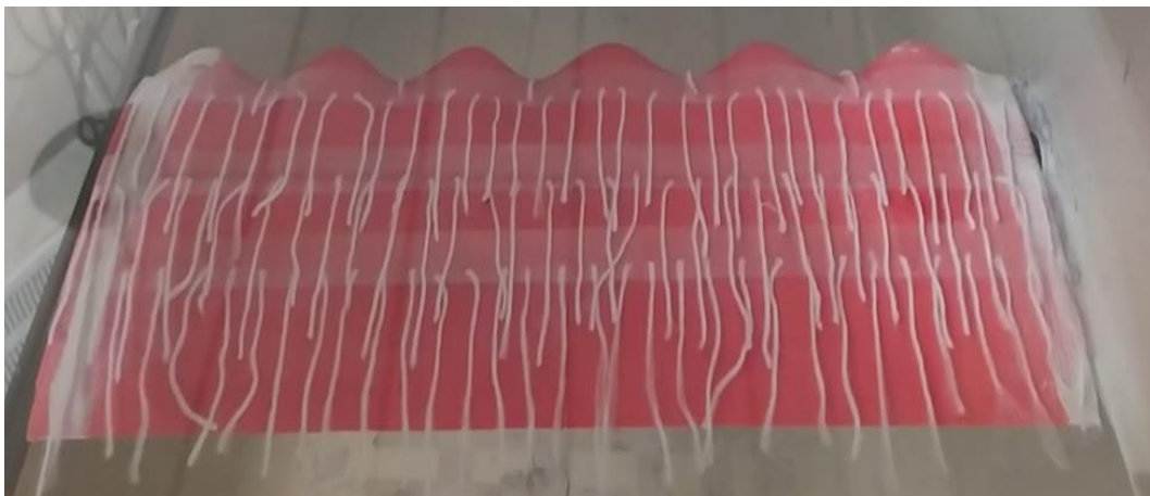
Figure 26. NACA 2412 (N6 \gamma 22 \lambda ) at \alpha=0^\circ
