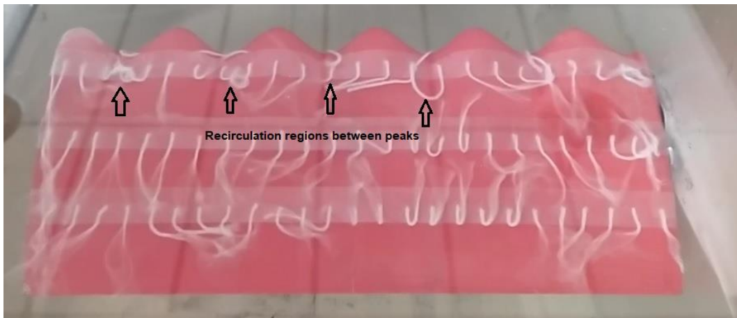
Figure 18. Recirculation regions between peaks of the wavy leading edge. Clark Y (C6 \gamma 22 \lambda ) at \alpha= 20^\circ
