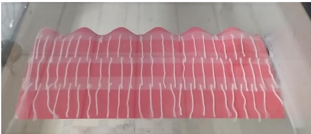
Figure 16. Flow attached to the surface. Clark Y (C6 \gamma 22 \lambda ) at \alpha= 0^\circ
