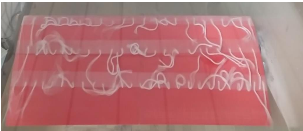
Figure 22. Flow totally separated. NACA 2412 at \alpha=15^\circ
