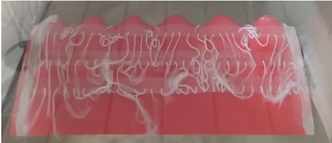
Figure 28. Stall of NACA 2412 (N6 \gamma 22 \lambda ) at \alpha=15^\circ
