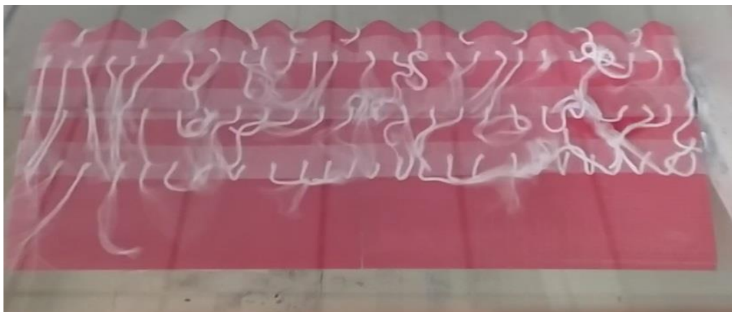
Figure 14. Flow totally perturbed. Clark Y (C3 \gamma 11 \lambda ) at \alpha= 20^\circ
