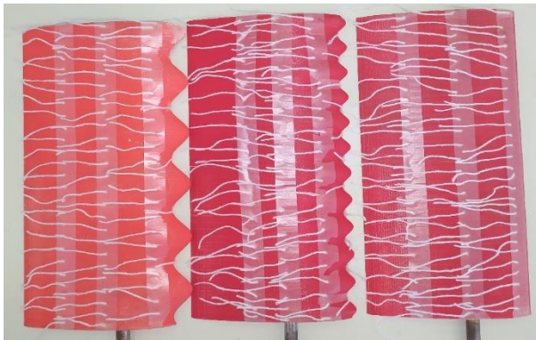
Figure 6. Wool tufts on the Clark Y upper surface.
