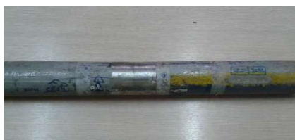
Figura 4 - CP 04, TP304L, Tubo + Tubo (Autor, 2017)
