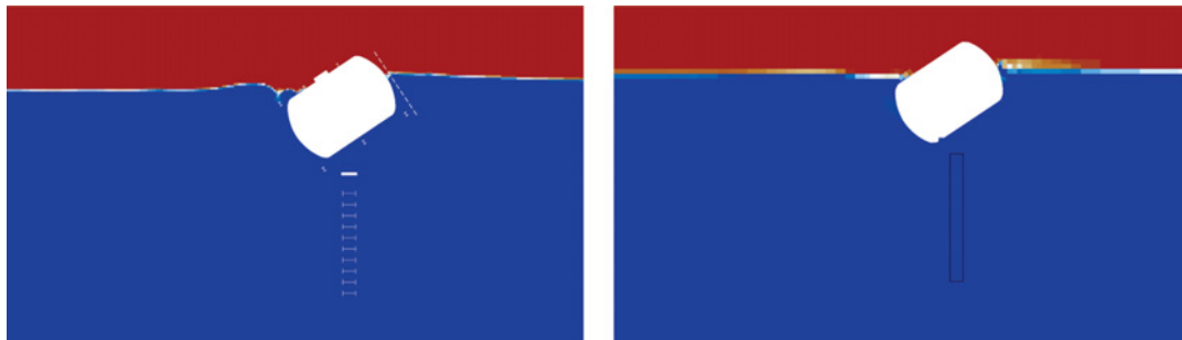
Figure 15. Comparative of VOF between complete (left) and simplified (right) model - v_a = 2.0 m/s and \beta = 0 deg
